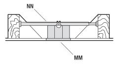
To hang your fan where there is an existing fixture but no ceiling joist, you may need an installation hanger bar (NN) (not included) as shown above.
